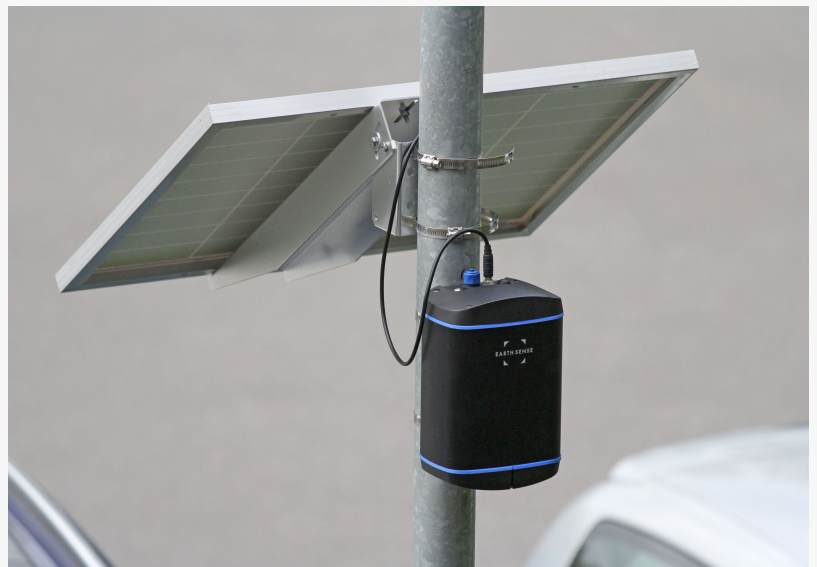
Zephyr® Air Quality Sensor Attached to Lighting Infrastructure.jpg
