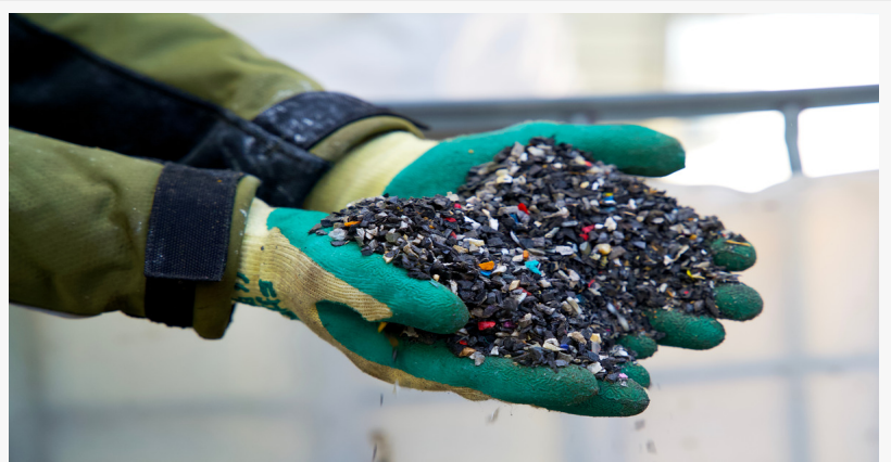
Granulated plastic waste on a recycling plant for plastics
