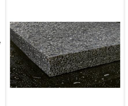
foams are used for thermal insulation in buildings, pipes, and packaging.
