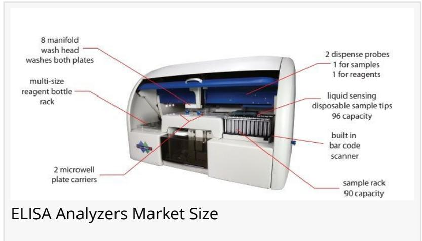
ELISA is an analytical biochemistry assay that utilizes a solid-phase enzyme immunoassay in order to detect the presence of a particular substance in a liquid sample. ELISA analyzers are automated instruments used in laboratories to carry out the ELISA test.
