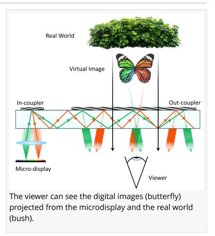
technology. AR enhances our perception and interaction with the environment by seamlessly blending projected virtual content with real-world scenes. Waveguide-based AR displays have emerged and developed as a key technology for wearable AR systems, enabling them to be lightweight and have a slim form factor while keeping high optical performance.
