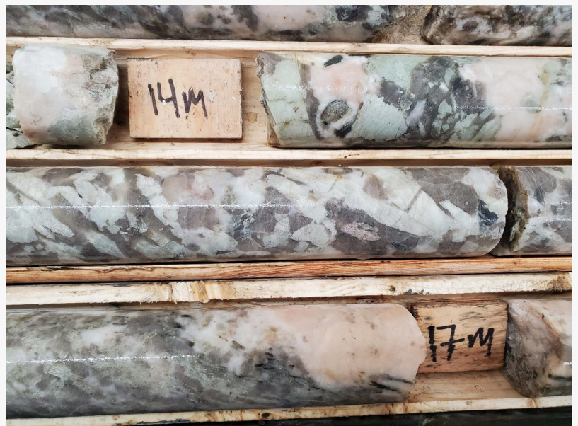
Shallow intersection of pegmatite hosting spodumene (pale green 'blades' in hole ZIG-23-01).
