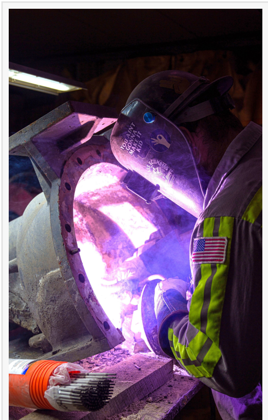
A Heidelberg Materials employee and student in the program uses the stick welding process on a piece of equipment during training at the plant in Union Bridge, Md.
