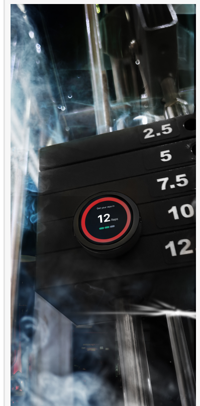
Rep2maX's rep counting device attached to weight stack counting reps
