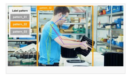
VP-Motion uses VisionPose, a highly successful proprietary engine that allows unparalleled accuracy when it comes to skeletal inference, or the act of deducing the skeleton of someone through camera footage. This is all done through AI, which means that markers are unnecessary, and all you need is any ordinary camera that can connect to your computer.
