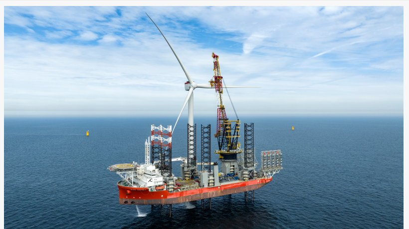
Cadeler wind turbine installation vessel
