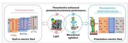
THE FORMED BUILT-IN ELECTRIC FIELD AND POLARIZED-INDUCED ELECTRIC FIELD AT THE INTERFACE OF HETEROJUNCTION TO PROMOTE CARRIER SEPARATION.
