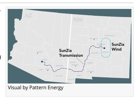
Once erected, SunZia Wind will be the largest onshore-wind project in the Western Hemisphere. It comprises more than 900 wind turbine generators from General Electric and Vestas in the state of New Mexico. SunZia Transmission, an 880 km ±525 kV high-voltage direct current (HVDC) transmission line, will transport the generated clean power from the wind-rich regions of the Midwest to high demand load centers in Arizona and California.
