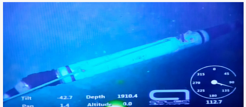
Image of one of the three SMART cable instrumented repeaters on the seabed following deployment. The repeater houses the Güralp seismometer and accelerometer.
