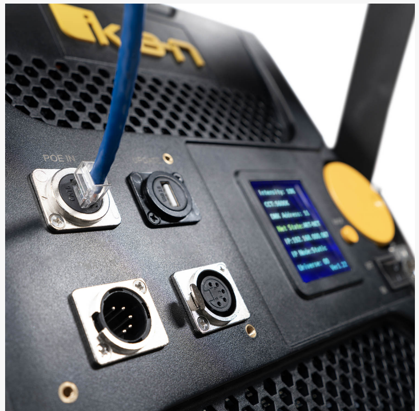
Lyra POE LED Lights use a single RJ45 cable for power and data.
