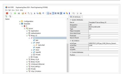
Complete IED tree in Engineering Base: For the first time, the attribute sets of the vendor-neutral IEDs can be filled directly in the engineering system in accordance with IEC 61850.
