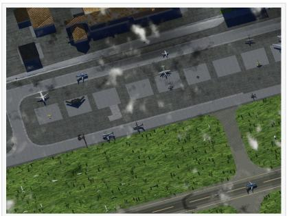
AgileView's synthetically generated image of an airport includes atmospheric conditions like clouds and shadows to help train the AI model, mimicking the way a satellite captures these features.
