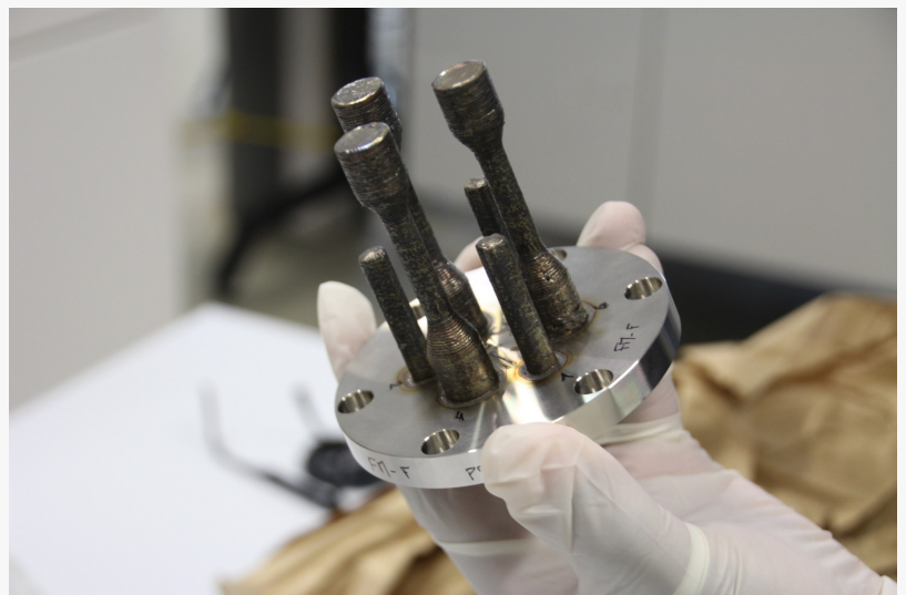
Samples produced by the Metal 3D Printer prior to launch to the space station. Photo courtesy of ESA.
