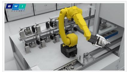
The robot auto-completes the material loading on the workstation and programs the module after the system has compared product information
