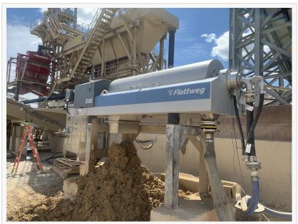
Efficient operation, robust design, and high purity output make German-made Flottweg decanters a multi-talent in the mining industry.
