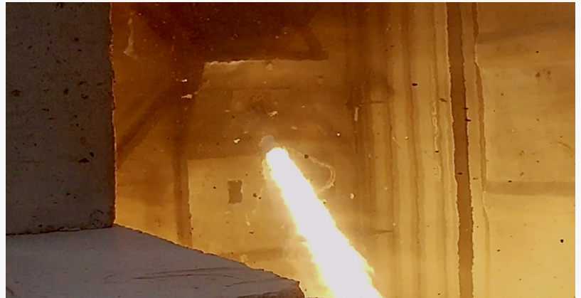
Image captured during one of NordSpace's recent tests of its flight ready, liquid bipropellant, rocket engine, the Hadfield-10.
