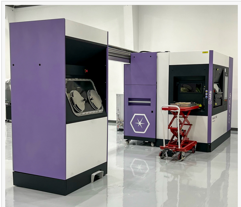
AddUp’s FormUp 350 Powder Bed Fusion machine onsite at Armadillo Additive’s new facility
