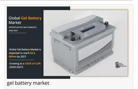
The gel battery contains a predetermined amount of electrolyte, which includes sulphuric acid and silica fumes. It falls under the category of valve regulated lead acid (VRLA) batteries and finds applications in various fields like electrification, hybrid power systems, navigational aids, mobile phones, motorcycles, camcorders, marine equipment, and more.
