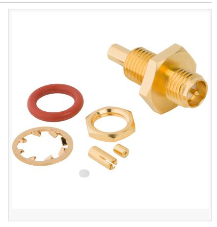
These RP-SMA front mount jacks are available in the straight configuration and feature a bulkhead design. They are constructed primarily with gold plated, brass while the contact is manufactured from gold plated, beryllium copper. The contact is soldered to the cable center conductor. The outer conductor works as an electromagnetic shield so the electrical signal transmitted on the center conductor is less susceptible to electromagnetic waves.
