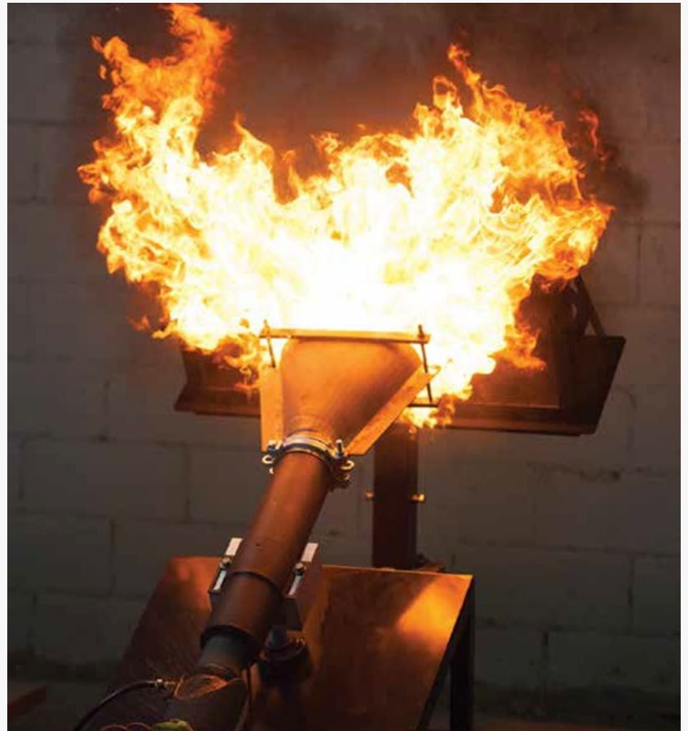
SGS flammability testing apparatus
