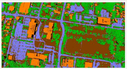
Subclassifications, a new training and custom classification feature in Global Mapper Pro v25.1, can be added to classifications to refine further the type of point feature with which it is being worked. Subclassifications are distinct in color and classi
