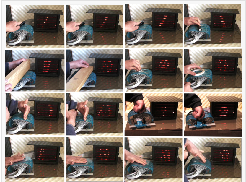
Low resolution 5 row OBD shape sensor prototype. Can digitize position, shape, weight, curvature, displacement, force, motion, pressure, timing, weight, etc.
