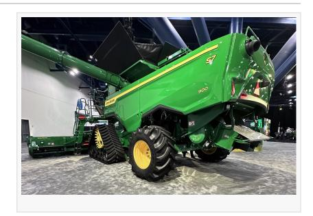
models - S7 600 with 367hp, S7 700 with 460hp, S7 800 with 540hp, and S7 900 with 617hp - boast powerful engines and advanced grain-handling and residue management features.
