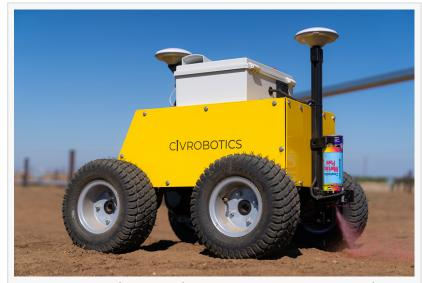
Leveraging Polaris Real-Time Kinematics Network (RTK), Civ's robot rovers can translate construction plans to real-world layout markings that are accurate to within less than a centimeter
