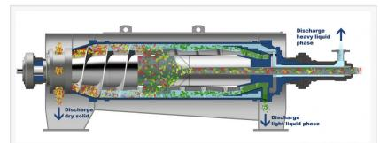
The centrifugal force generated enables the Sorticanter® to separate different types of plastic from each other. This enables operators to achieve the highest possible purity of plastics.
