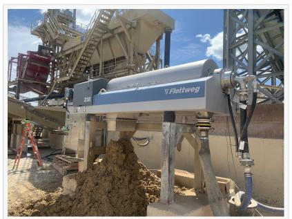
To save up to 90% pond space or even more, a decanter centrifuge combined with a clarifier / polymer dosing unit is a very affordable and effective solution.
