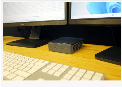
The NUC DECK N95 also provides excellent visual capabilities, supporting triple-display with HDMI 2.0b and DP 1.4a (through Type-C) up to 4096x2160@60Hz.
