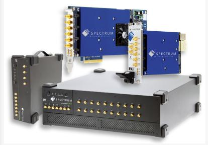
23 different AWGs are able to use the new DDS firmware option. They offer 16-bit resolution, up to 1.25 GS/s speed and up to 32 channels.
