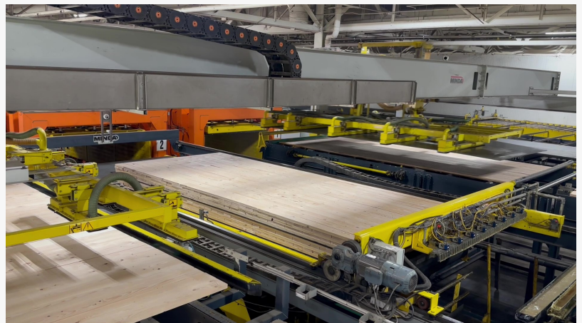
Eastern hemlock CLT being manufactured at Sterling Structural
