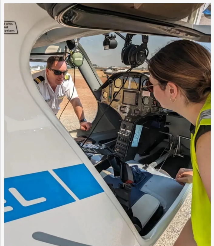
Electro Instructor Gareth Lloyd shows a student the avionics inside the Pipistrel electric sports aircraft
