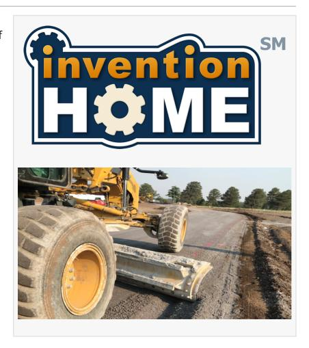
aggregate base out from finished grade before asphalt or concrete is placed, ensuring there is a proper edge to prevent failure or deterioration. Ultimately, the attachment saves time and money on asphalt and concrete yields and labor costs.
