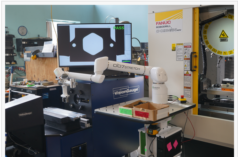
The new VisionGauge Automation Module interfaces directly with external production machinery and cell controllers.
