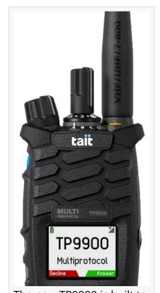
The new TP9900 is built to speak in three radio "languages" (P25 and DMR digital as well as in analog) and can access a wide spectrum of radio frequencies. In industry-speak it's called multiprotocol, multiband.
