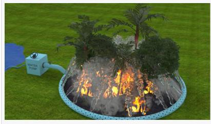
with ring holes throughout. Users can connect the hose to a water pump and water source. Inside the fire hose is a long sliding valve that is adjusted. It can be closed when filling in the fire hose with water and slid to open when starting the sprinkler, using the valve switch. Anchors are placed on the side of the fire hose to hold down the sprinkler fire hose due to pressure from the water pump.
