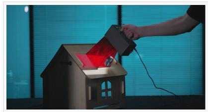
The Longer Nano handheld portable engraving machine is carving
