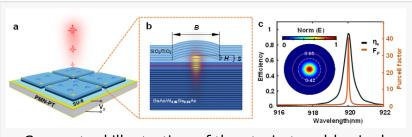
a, Conceptual illustration of the strain tunable singlephoton source. b, Structure of the integrated FP microcavity and electric field distribution of fundamental mode. c, 3D-FDTD simulation design.
