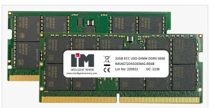
DDR5 memory modules in commercial and industrial temperatures from Intelligent memory
