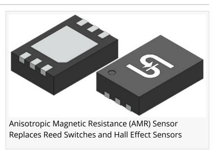
hall effect sensors in industrial applications. The <u>TSHA2101</u> is an integrated system-on-chip (SIP) requiring little to no added circuitry. Its omni-polar design automatically detects a horizontal magnetic field of either polarity. When positioned to detect a magnet located on a linear or rotational element, the TSHA2101 acts as a non-contact switch with low power consumption,
