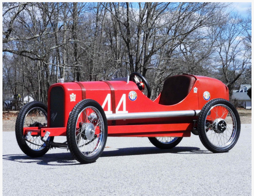
1924 Alpha Romeo half-scale Shriners parade P2 go-cart racer with a steel frame and a wood and spray foam body, and fitted with a gas-powered Honda 200 engine (est. $2,000-$6,000).
