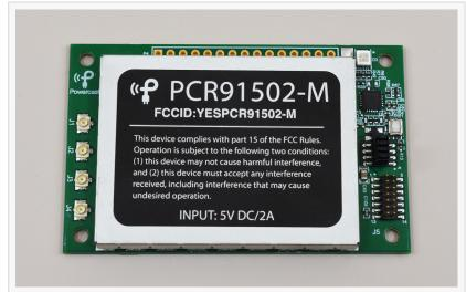
Ruggedized module, a finalist in RFID Journal LIVE's Best New Product Awards, costs less and withstands more extreme temperatures, -40°C to +85°C, than typical modules operating from -20°C to 70°C
