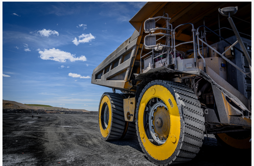
Close up on of Mining Truck with the New Airless Tire Technology
