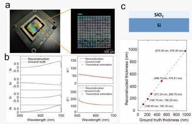
The metasurface array-based system for single-shot spectroscopic ellipsometry measurement.
