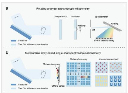
a, Schematics of a conventional spectroscopic ellipsometry system. b, Schematics of a metasurface array-based single-shot spectroscopic ellipsometry system.
