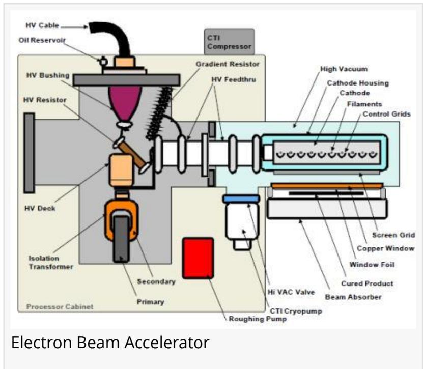
Electron Beam Accelerator
