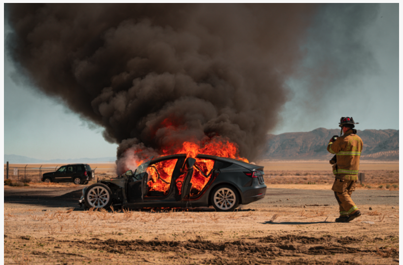
E-FireX test on fully involved Tesla with firefighter testing heat reading
