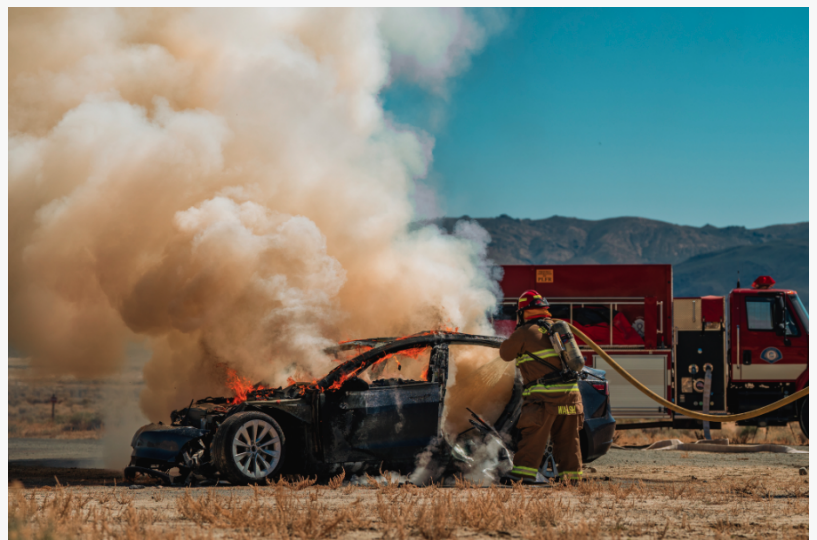
E-FireX test on fully involved Tesla extinguishing fire using 200 gallons of water and E-FireX’s TRPL-E™
