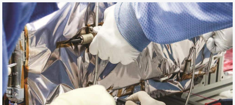
Dunmore's multilayer insulation (MLI) films in use
