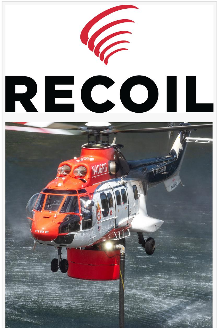
Recoil Aerospace announces the successful certification of its T1000-E Aerial Fire Suppression System (AFSS) by the Federal Aviation Administration (FAA) for installation on Airbus Super Puma series helicopters.
